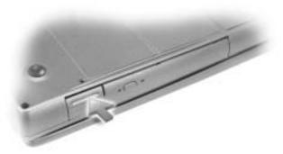
**3** Pull the device out of the module bay.
